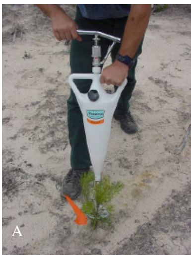
Kioritz (A) and PTM spot gun (B) soil injectors for application of PTM solution. (Photos by Don Grosman & Harold Quicke, BASF); SilvaShield Forestry Tablets (C) (Photo by Don Grosman).
