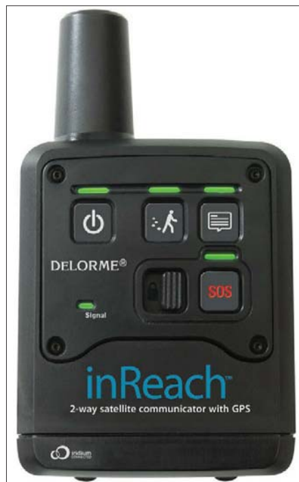
DeLorme's inReach satellite communicator, paired with a DeLorme EarthMate PN-60w GPS receiver or an Android phone, offers two-way messaging anywhere on Earth.
